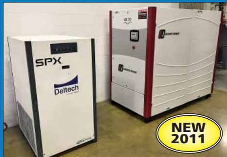
100-HP Gardner Denver Model V545-70A Rotary Screw Air Compressor
