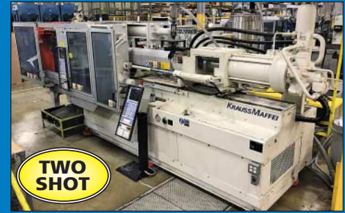
331 Ton x 33.6 Oz. Krauss Maffei Model 300-1900C2 PIMM w/ SP390 Bolt-On Injection Unit
